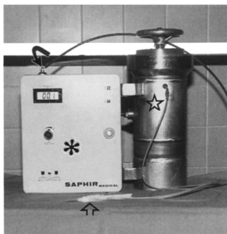
Fig. 1 Water-jet dissector: ➔ pressurised gas admission, ☆ pressurised airtight steel chamber containing the sterile water pouch, ➔ electronic system control, ➔ hand piece with nozzle delivering a 0.2-mm-diameter water jet
